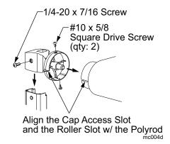
Figure 4. Attaching the Idler End Plug.
