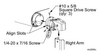
Figure 2. Attaching the Manual Crank.
