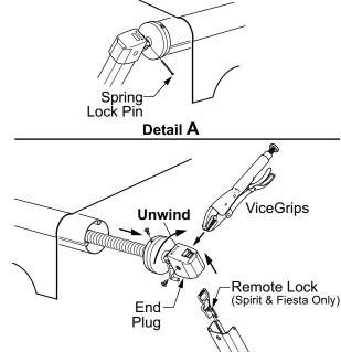
Figure 1. Removing the RH Spring.
