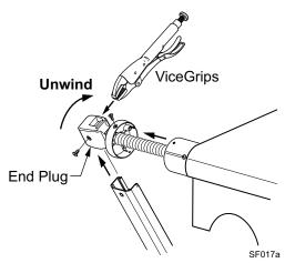
Figure 3. Removing the LH Spring.
